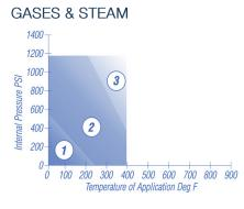
In area ① the gasket material is suitable using common installation practices subject to chemical compatibility.
