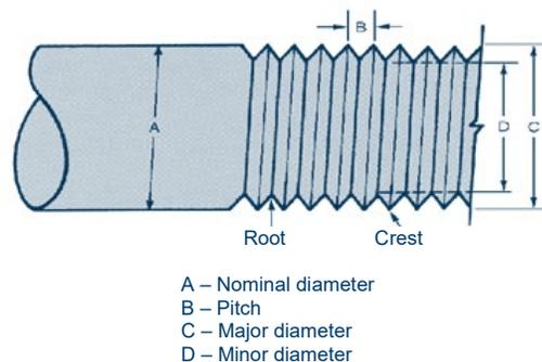
In the above figure, the arrows point to the root and the crest of the threads. The pitch of the thread is the distance from the crest of one thread to the crest of the next thread. This measurement is used to determine the number of threads per inch, or millimeters per thread, data that are usually supplied by the fastener manufacturer. The one most frequently used term in designating the size of a bolt or screw fastener is its nominal diameter.
